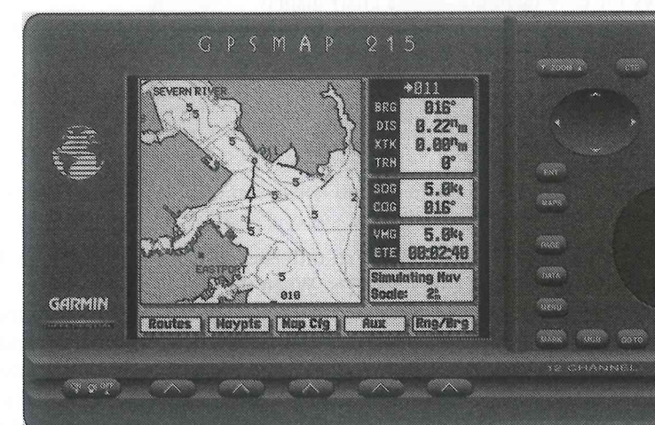
Figure 5.30 Front panel of the Garmin GPSMAP 225 system showing operator controls and a sample navigation map generated in the simulation mode. (Reproduced courtesy of Garmin.)
