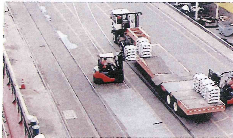
✓ Handling pre-slung, bundled, medium-size ingots. Loading on a trailer for further storage in a warehouse
