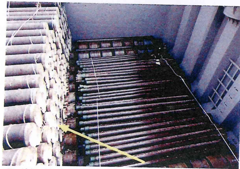
✓ Lightweight pipes loaded over HRC in a lower stow. The ship does not have side under-coaming areas
