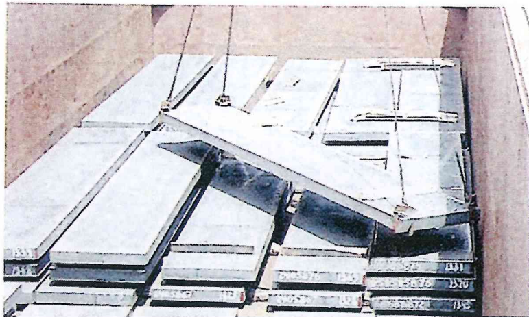
✓ Loading of slabs in progress. Good, square, hardwood dunnage is used between the tiers
