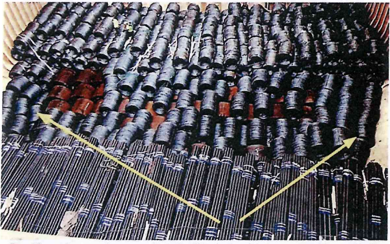
✘ The under-coaming stow of WRIC will be impossible to access with a vertical plumb of the crane. A forklift truck to provide access to the WRIC cannot be utilised
