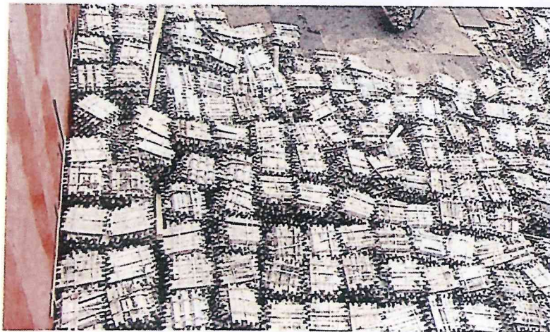
✗ Poor stowage. Cargo stow is not levelled
