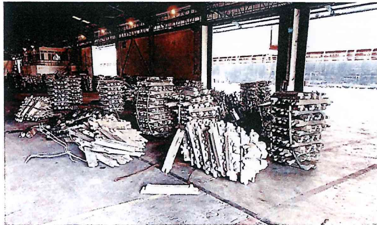
✘ Improper bundling. Ingot bundles loose in the warehouse
