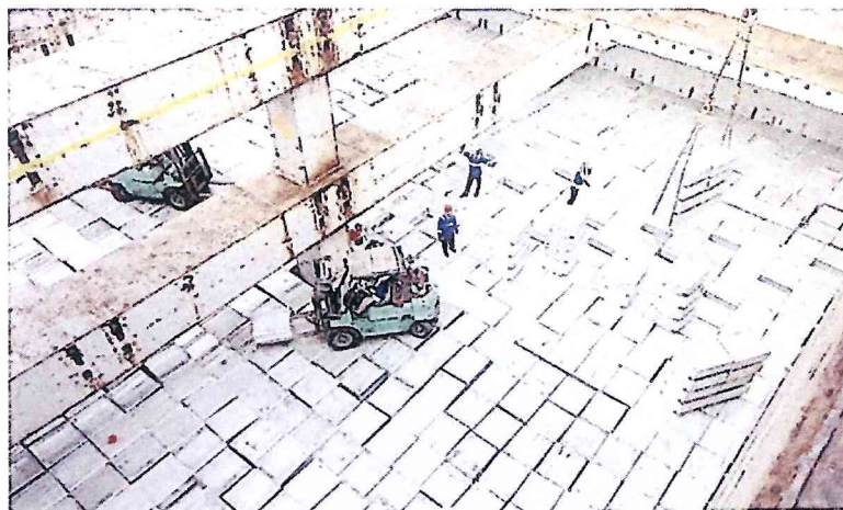
✓ The use of a forklift truck for the discharging of T-ingots from a box-type cargo compartment. The stow is full and compact
