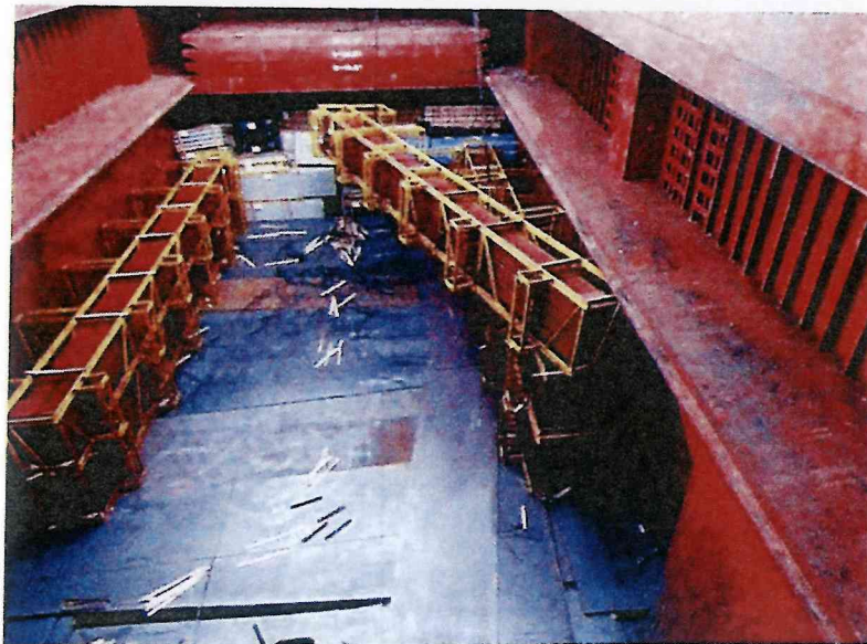
✓ Loading of palletised structural steel over steel plates. The stow of plates is properly levelled
