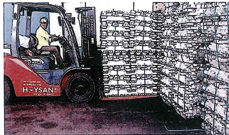
✓ Discharging small-size palletised ingots with the use of a forklift truck
