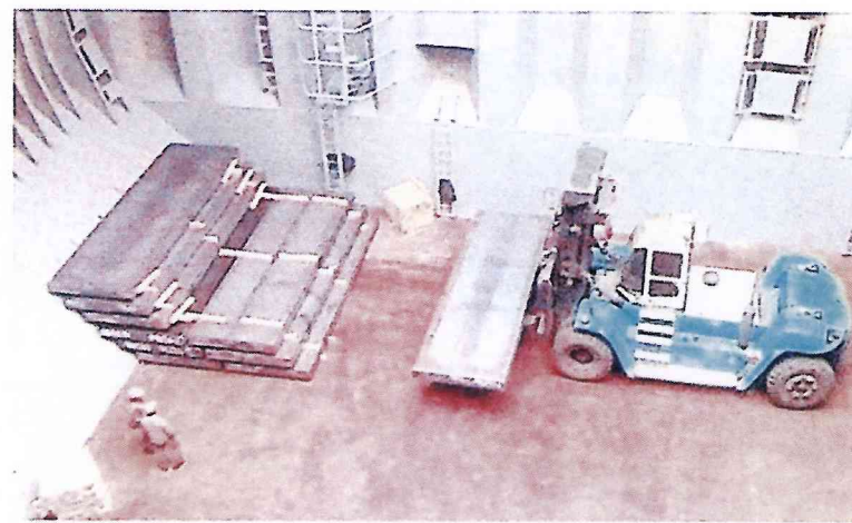
✓ A fore-and-aft loading of slabs. Proper use of dunnage
