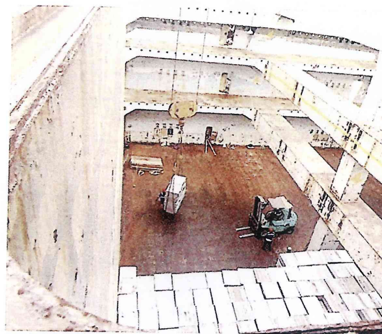
Handling aluminium T-ingots with chain slings
