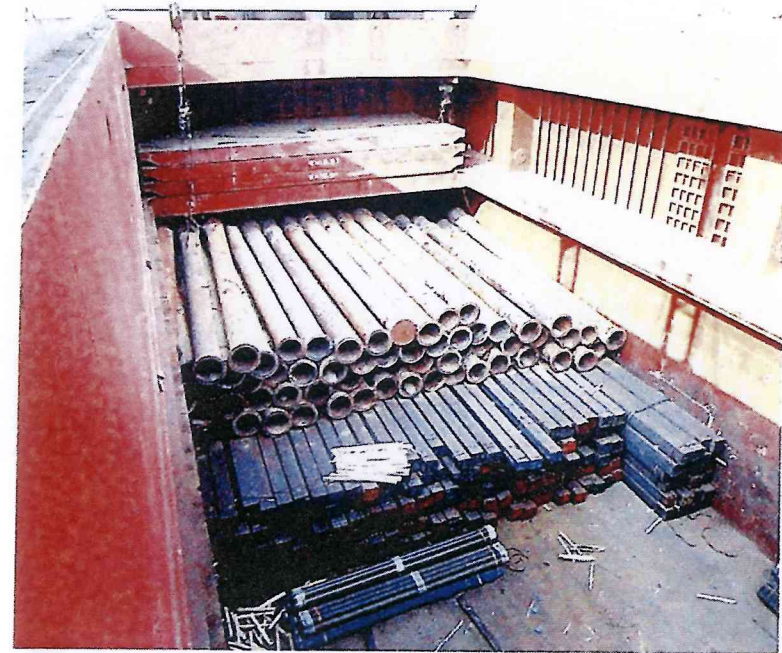
✓ Pipes loaded over structural steel cargo in a box-shaped cargo hold
