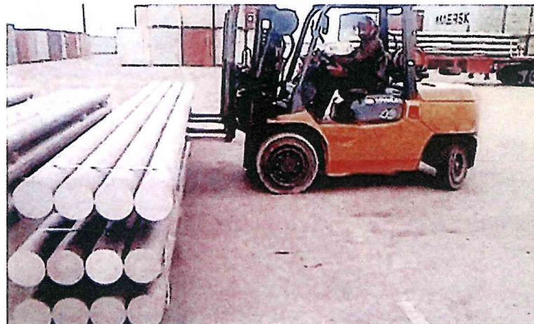
✓ Bundled, long, round aluminium billets handled with a forklift truck and prepared for loading
