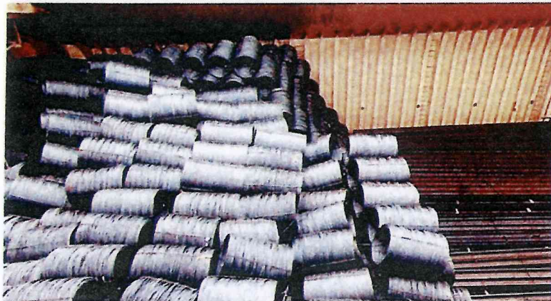
X Insufficient dunnaging and lashing of the WRIC stow over the structural steel stow
