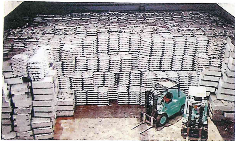
✓ Use of forklift trucks for discharging bundled ingots and T-ingots from a box-type cargo compartment
