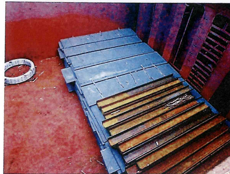
✓ Dunnage and lashing properly prepared for the stow of structural steel products
