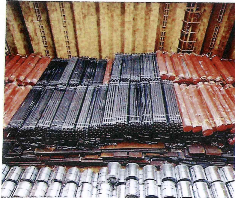
✓ Pipes may be loaded over some structural steel, such as H-beams and I-beams. In this photograph, the H-beams are also loaded on top of steel plates
