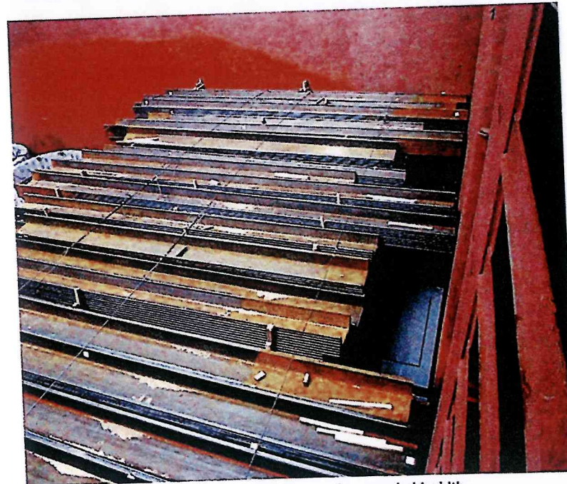
✓ Structural steel reasonably lashed across the cargo hold width
