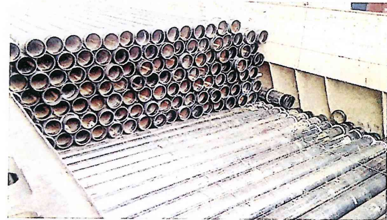
✓ Swaged pipes loaded in an athwartships and longitudinal stow. Note that rope grommets are used at both ends to protect the swage. No dunnage was used
