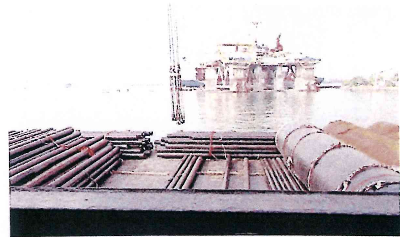
The pipes discharged with hooks to barges. The pipes should be pre-slung
