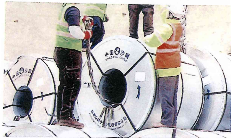
✓ Braided wire sling is passed through the coil in preparation for discharging
