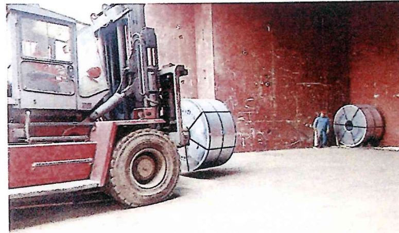
✓ Use of a forklift truck equipped with a pole to handle coils under the coaming area
