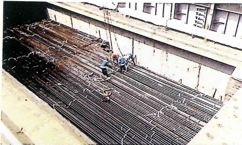
✓ Pre-slung pipes. The stevedores use tipping hooks to prepare the single basket lift for discharging
