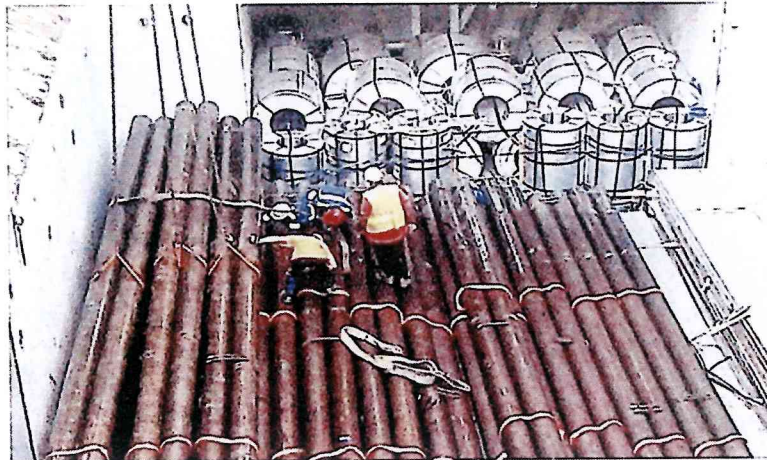
✓ Pipe bundles being tipped by sorting hooks at Jurong Port, while the nylon lifting slings are positioned underneath. The pipes are pre-slung for tipping
