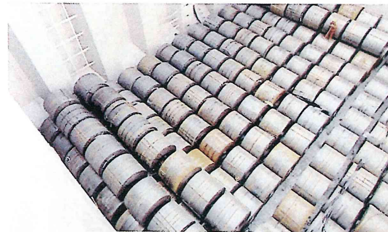
✓ Box-type cargo compartment. A single-tier stow of HRC without locking coils. The second tier is not complete
