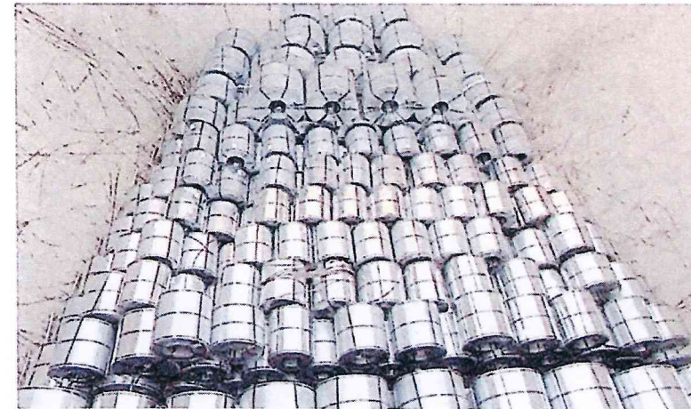
✅ Correct loading and pyramid stowage of CRC in fore-and-aft direction in hopper-type cargo hold with flaring of the coils
