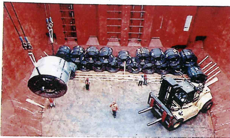
✘ Loading of HRC in a hopper-type cargo hold. HRC are generally heavy and three rows of dunnage are not sufficient
