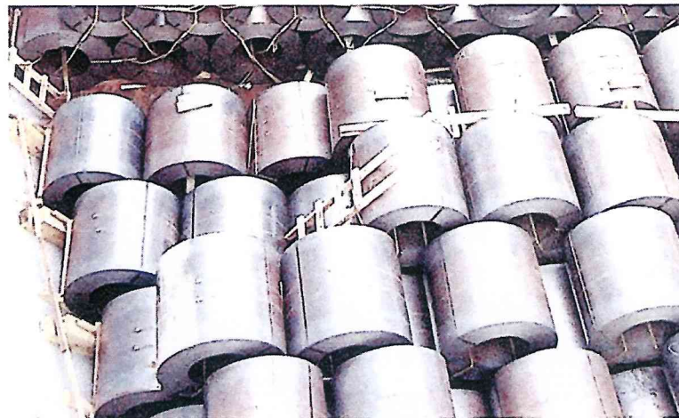
✔ Good storage of coils with shoring dunnage at the bulkhead and safety access to the top tiers of coils
