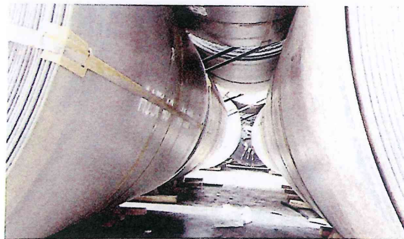
✘ Insufficient space for a locking coil. No chocking dunnage is used to prevent the coils from shifting
