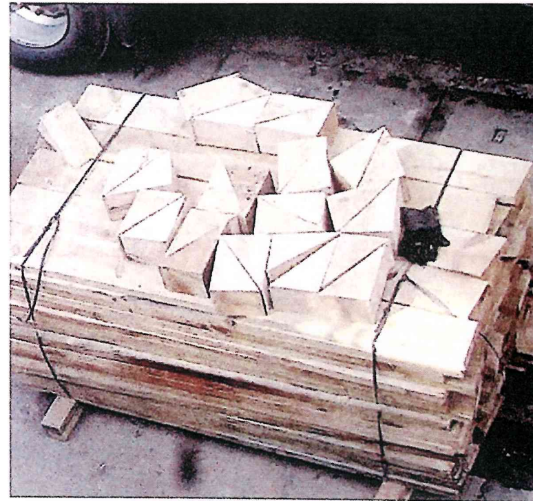
Dunnage boards and wood wedges prepared for the loading of steel coils
