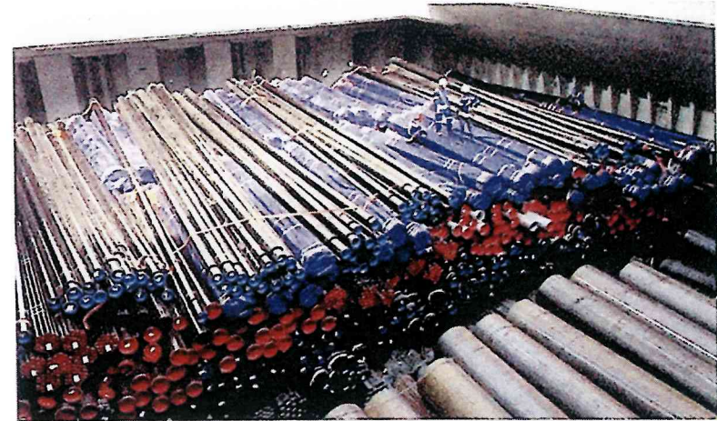
✗ A loose stow of mixed size and bundled pipes, making discharge difficult, dangerous and slow. For mixed size pipes, pre-slinging is required
