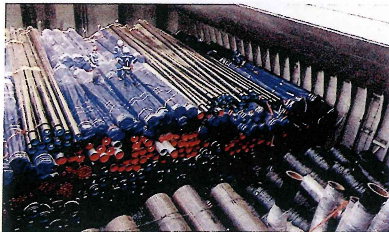
✗ Stow of various bundled and single pipes. The stow is not level. No dunnage is used. Pre-slinging with nylon web slings is required for such a stow
