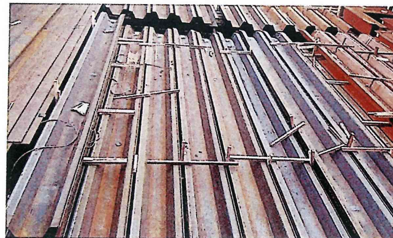
✓ Good level stows with vertical dunnage wedges
