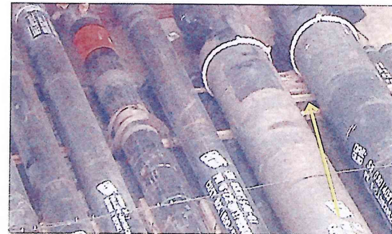
✓ Lashed stow of various diameter pipes. Wires used for lashing. Note the dunnage between the tiers
