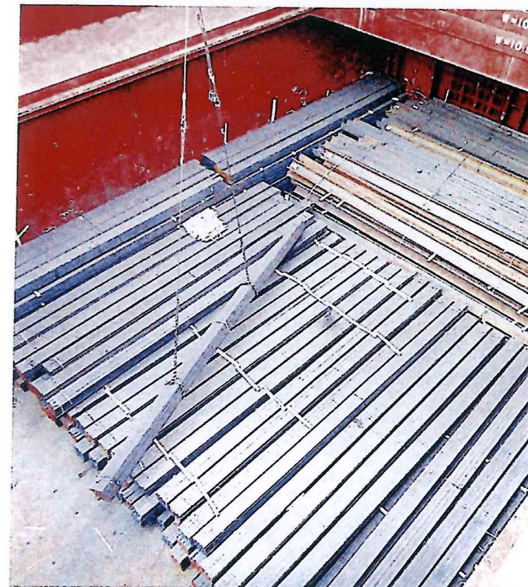
✓ A good, even stow of structural steel bundles with dunnage between the tiers to assist the discharge operation
