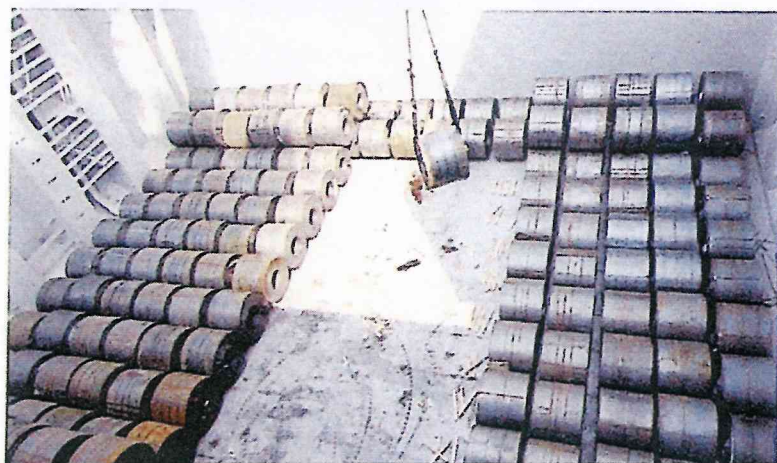
✓ Handling of HRC with long braided wire slings without a spreader, which is acceptable. This is not acceptable for CRC
