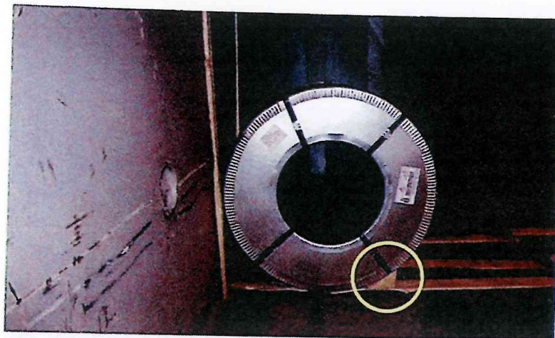
✘ First tier of coils. Correct place for the wooden wedge on the dunnage plank, but incorrect positioning with the right angle down. Dunnage too thin
