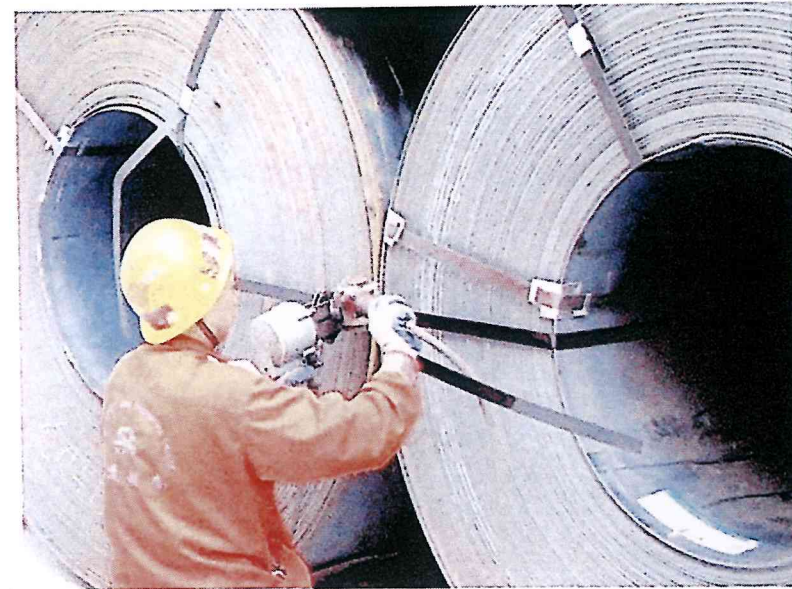
Tightening of steel strapping bands with a pneumatic tool. For coils of the size in the photograph, double metal straps should be used for lashing
