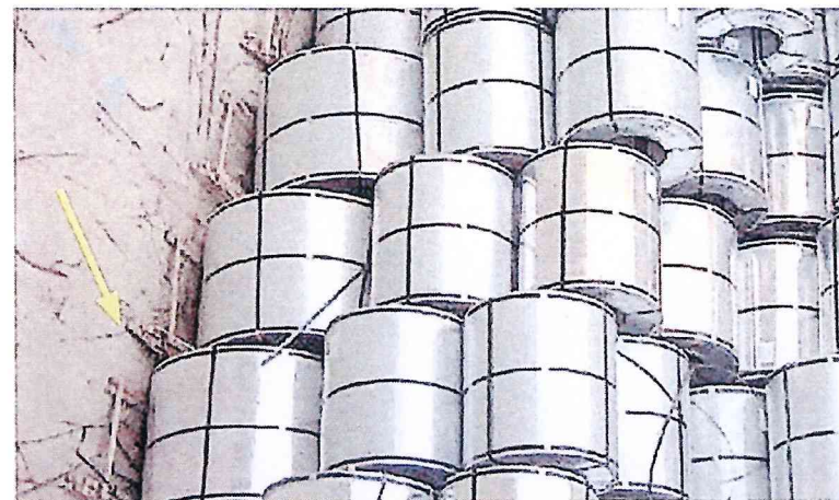
❌ Insufficient securing of the dunnage for shoring in one block. Shifted dunnage during the passage
