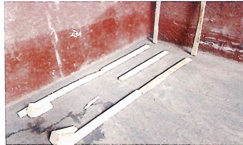
✗ Incomplete dunnage laid for the loading of coils
