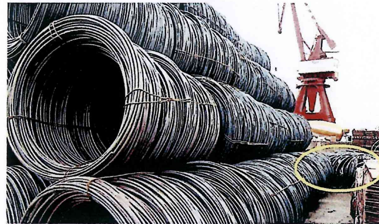
X Unprotected coils in open storage before loading. Note the unwound coil highlighted in yellow. Such WRIC should not be accepted for loading
