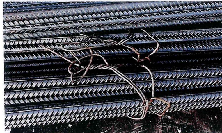
✗ Lifting bundles by the bundling wires can lead to loosened bundles and/or broken straps, increasing the difficulty for discharge and the risk of damage
