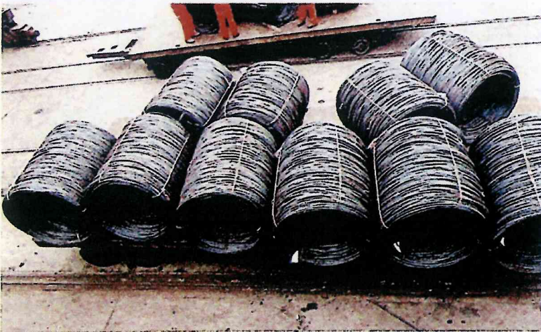
X Unprotected coils brought to the ship by trailer. Only four single wire rod bundles have been applied
