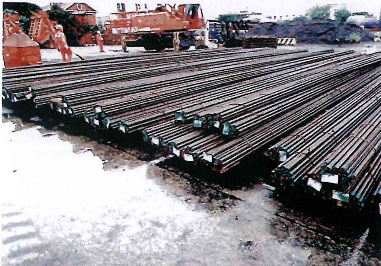
Rebar in open storage prior to shipment and showing signs of corrosion
