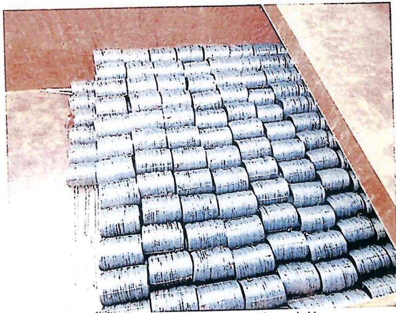
WRIC being stowed across the full width of a box-shaped cargo hold
