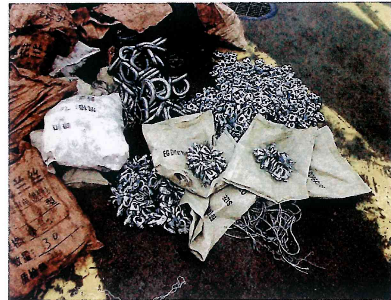
Bulldog grips and additional 'D' rings for cargo lashings
