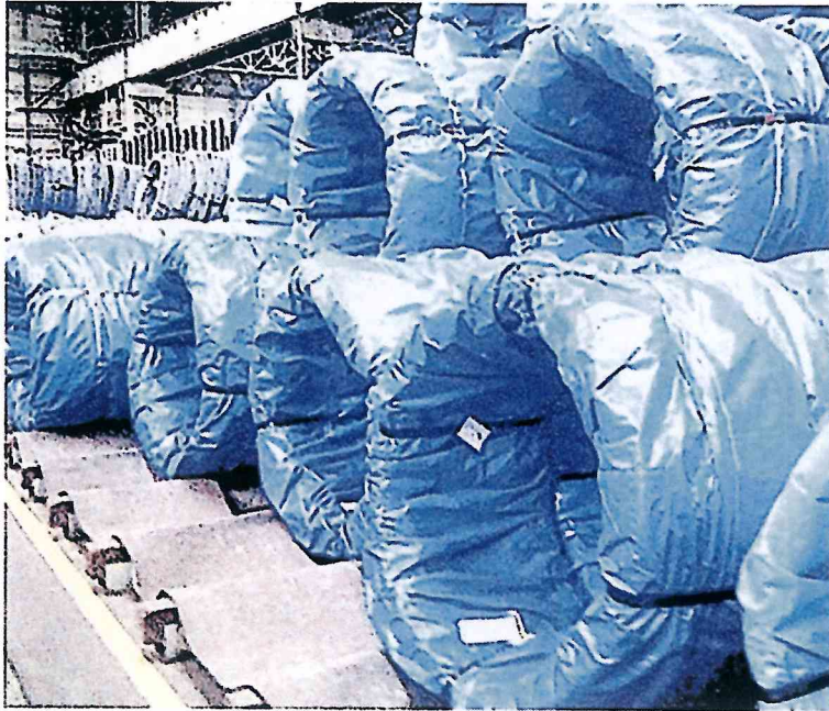
✓ Partially protected WRIC secured with four strapping bands
