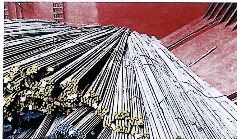
✘ 12 metre long rebar in the under-coaming space of a hopper-type bulk carrier. No dunnage. The stow is not levelled
