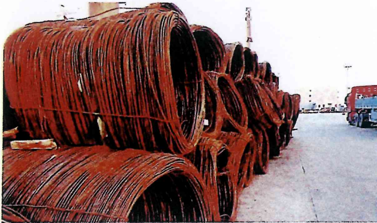
X Rust-covered, unprotected coils in open storage. The coils are damaged and the securing bands are loose. These coils will not make a tight and secure stow
