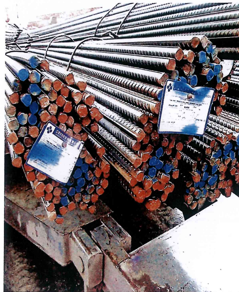
Bundling wires along the length of the bundles are not designed for lifting, but can be used for tipping
