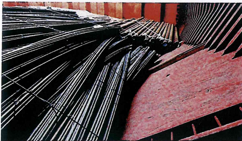
✘ Shifted cargo at the discharging port. Bad pyramid stow of 12 metre long rebar without dunnage. Shifting of the rebar inside the under-coaming space
