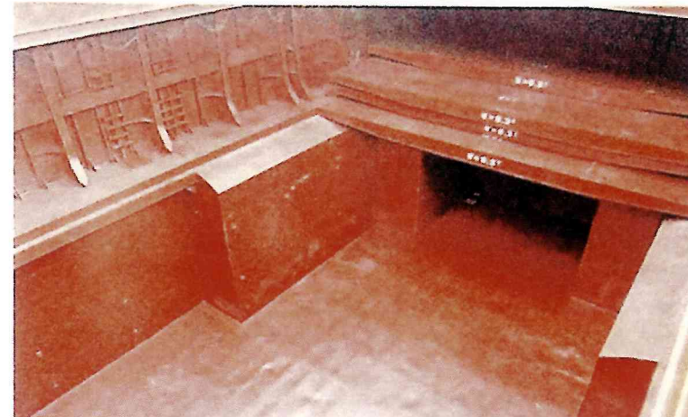
✓ A cargo ship with box-shaped cargo holds and pontoon 'tween deck ready for loading
