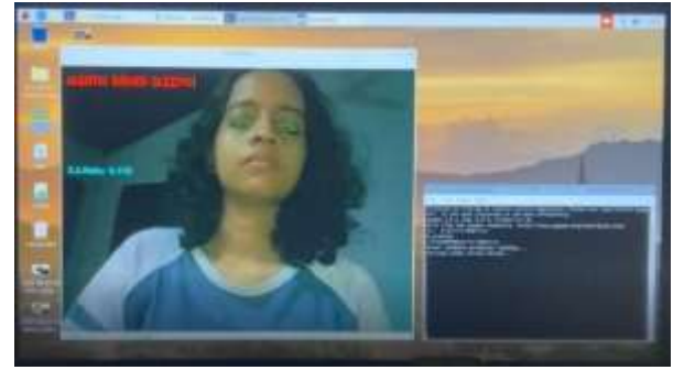
Figure 10 Determining sleepiness using Eye Aspect Ratio
