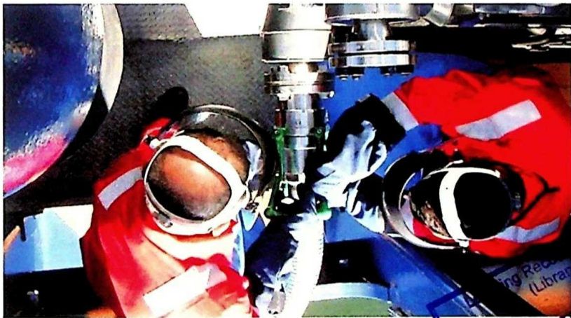
Hose connected to ship's bunkering manifold (image courtesy of Harvey Gulf International Marine)
