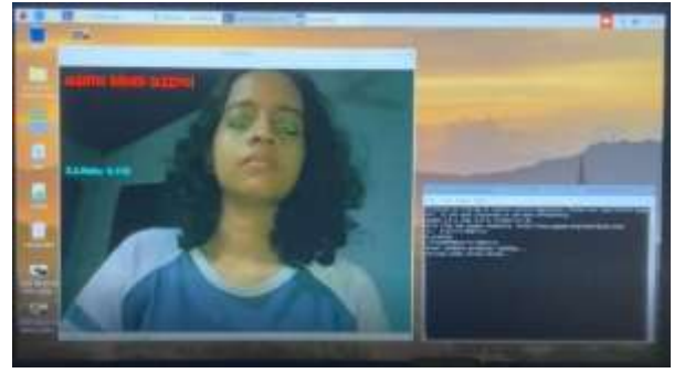
Figure 10 Determining sleepiness using Eye Aspect Ratio
