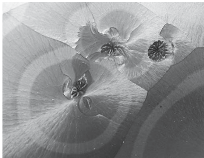
FIGURE 21.15 Illustration of spherulitic crystallization in a glass.
