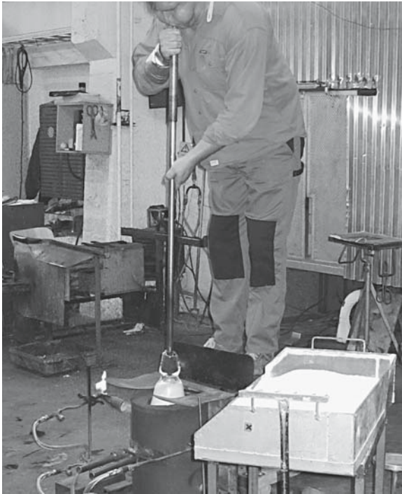
FIGURE 26.10 Demonstration of blowing glass into a mold. Note the worker's bench, the annealing burners, and the box of frit.
