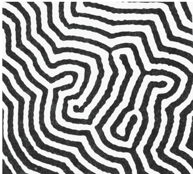
FIGURE 33.19 Domain pattern in a YIG thin film revealed by the Faraday effect. The stripes are 12\ \mu\text{m} wide.
