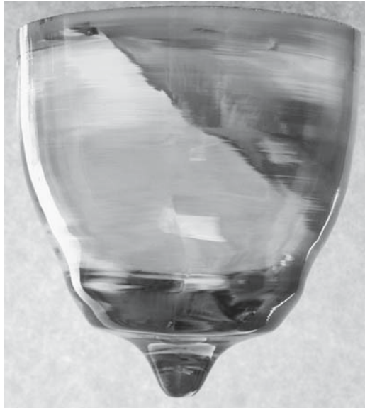
FIGURE 29.4 Lower part of sapphire boule grown by the Cz technique, the boule was 100–150 mm diameter; 300 mm long.
