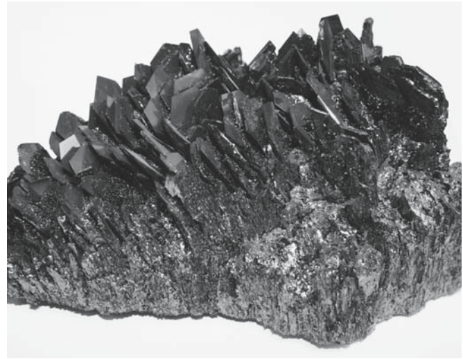
FIGURE 19.7 SiC produced by the Acheson process.
