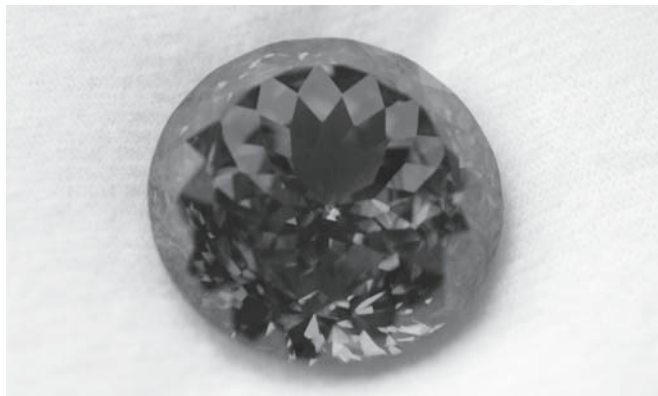
FIGURE 36.29 A single-crystal of RE-doped as-grown synthetic CZ. (Diameter = 2.5 cm).
