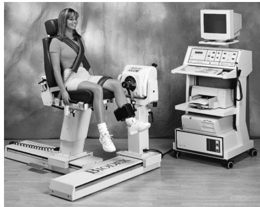
Figure 1.5. A computerized testing and exercise dynamometer by Biodex. The speed, muscle actions (isometric, concentric, eccentric), and pattern of loading (isokinetic, isotonic) can be selected. Image courtesy of Biodex Medical Systems.
