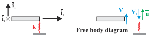
Fig. 16.8. Boundary conditions for an edge with a linear spring.
