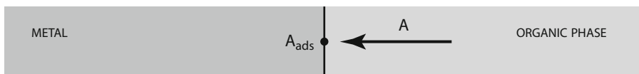
Figure 2.9 - Diagram of the adsorption reaction of a molecule A at an interface with a metal
