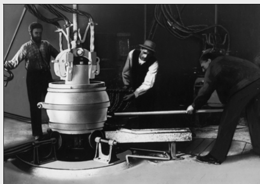
First electrolysis cells in Froges in 1889
