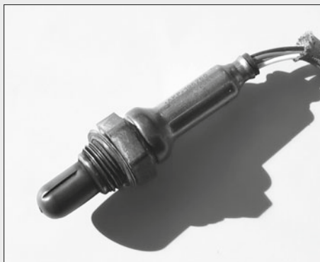
Photograph of a lambda sensor extracted from a car after use
