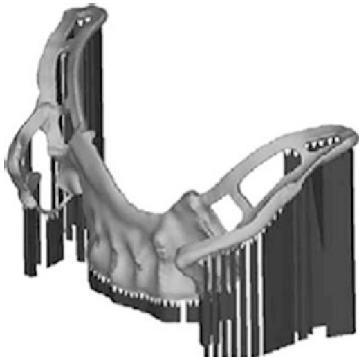
Fig. 14.4 Breakaway support removal for (a) an FDM part (courtesy of Jim Flowers) and (b) an SLA part (Courtesy Worldwide Guide to Rapid Prototyping web site. © Copyright Castle Island Co., All rights reserved. Photo provided by Cadem A.S., Turkey)
