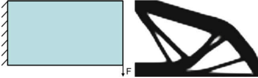
Fig. 17.18 Simple topology optimization example
