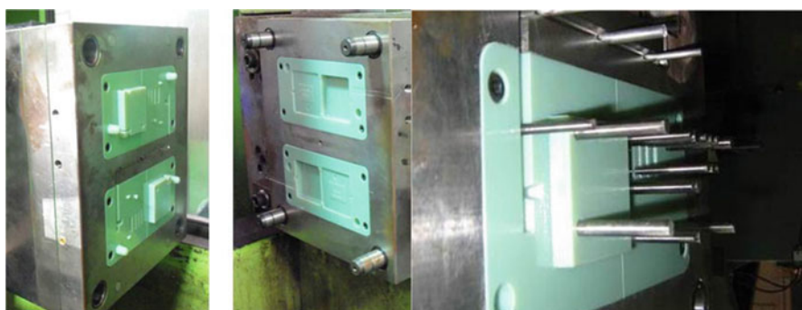
Fig. 18.3 Polyjet inserts for a two cavity mold set, showing a close-up of the ejector pins (courtesy Stratasys)
