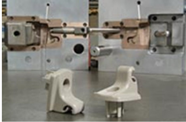
Fig. 18.4 A direct metal laser sintered tool set, with two parts that have been molded from them
