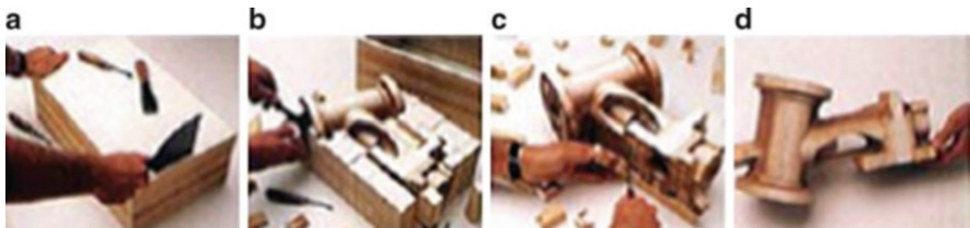
Fig. 14.2 LOM support removal process (de-cubing), showing: (a) the finished block of material; (b) removal of cubes far from the part; (c) removal of cubes directly adjacent to the part; (d) the finished product (Courtesy Worldwide Guide to Rapid Prototyping web site © Copyright Castle Island Co., All rights reserved. Photo provided by Cubic Technologies.)
