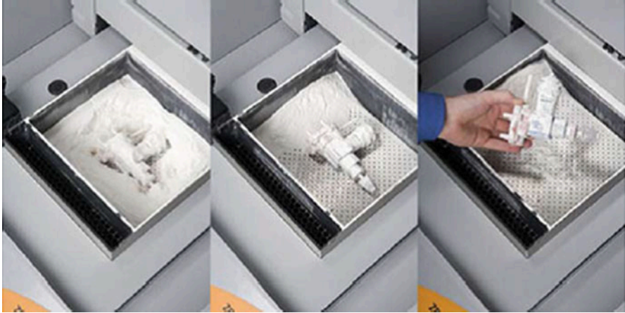
Fig. 14.1 Automated powder removal using vibratory and vacuum assist in a ZCorp 450 machine (Courtesy Z Corporation)
