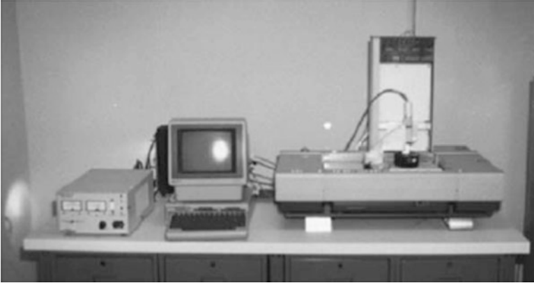
Fig. 2.7 The first AM technology from Hull, who founded 3D systems (photo courtesy of 3D Systems)
