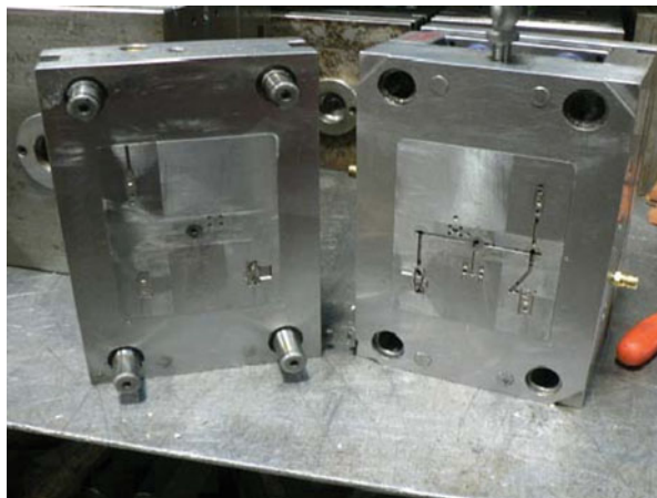
Fig. 18.2 A core/cavity mold set showing a central injection point and channeling to regions where 5 different parts are formed in one cycle
