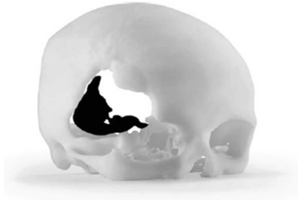
Fig. 6.4 A medical model made using extrusion-based AM technology from two different color materials, highlighting a bone tumor (courtesy of Stratasys)
