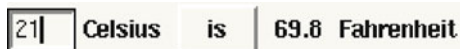
Fig. 4.1 Screen dump of the graphical interface for a Celsius to Fahrenheit conversion program. The user can type in the temperature in Celsius degrees, and when clicking on the is button, the corresponding Fahrenheit value is displayed
