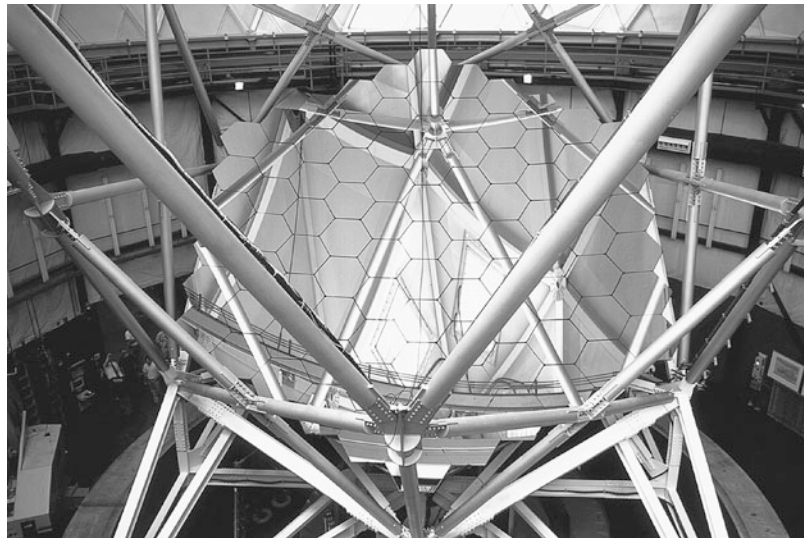
Fig. 3.20 The mirror of a telescope can be made up of several smaller segments, which are much easier to manufacture, as in the Hobby–Eberle Telescope on Mount Fowlkes, Texas. The effective diameter of the mirror is 9.1 m. A similar telescope is being built in South Africa. (Photo MacDonald Observatory)
