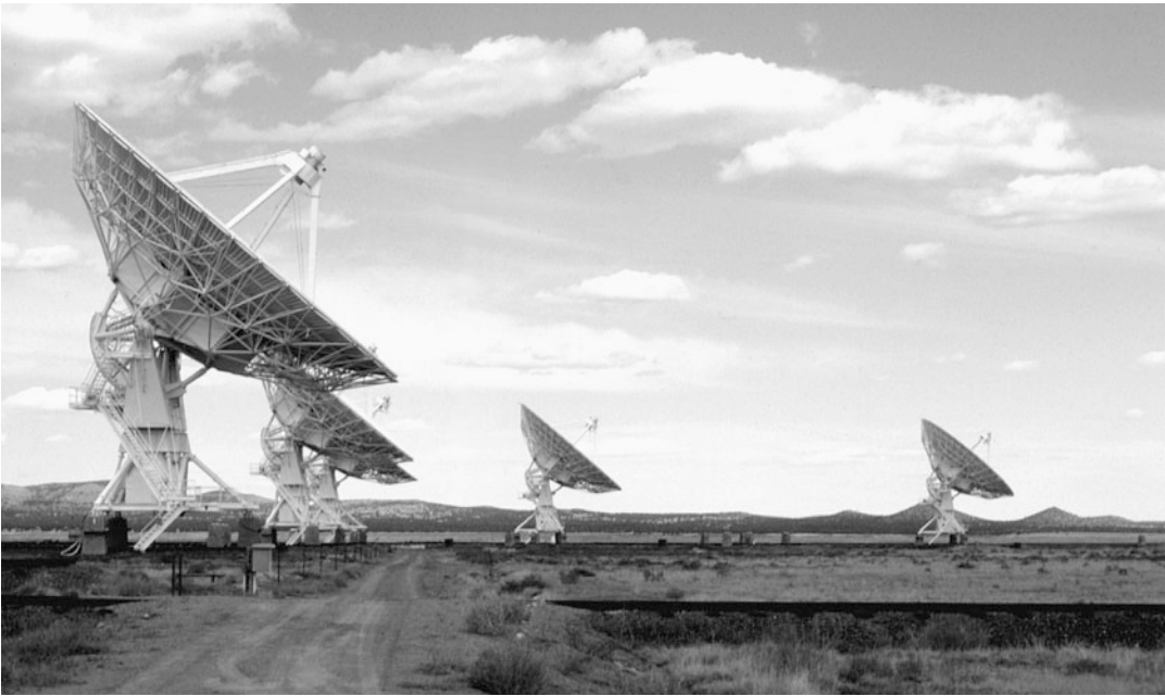
Fig. 3.34 The VLA at Socorro, New Mexico, is a synthesis telescope consisting of 27 movable antennas
