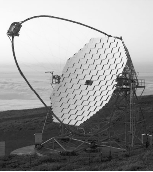
Fig. 3.35 The MAGIC telescope on La Palma in the Canary islands observes the Cherenkov radiation produced by gamma rays. (Photo Robert Wagner, Max Planck Institut für Physik)
