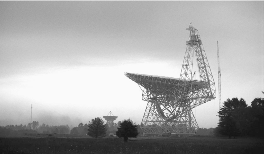
Fig. 3.30 The largest fully steerable radio telescope is in Green Bank, Virginia. Its diameter is 100 \times 110 m. (Photo NRAO)
