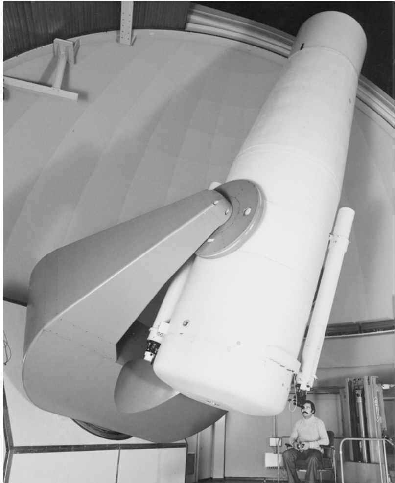
Fig. 3.16 The large Schmidt telescope of the European Southern Observatory. The diameter of the mirror is 1.62 m and of the free aperture 1 m. (Photo ESO)
