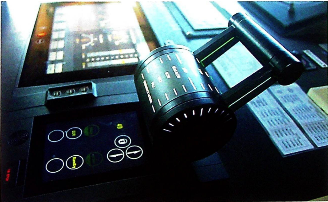
A modern main engine telegraph and control panel
