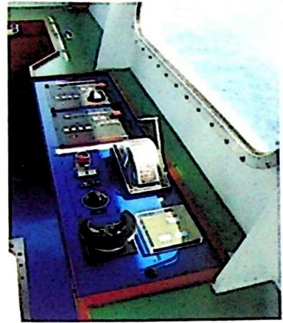
A mini wheel at the bridge wing manoeuvring position
