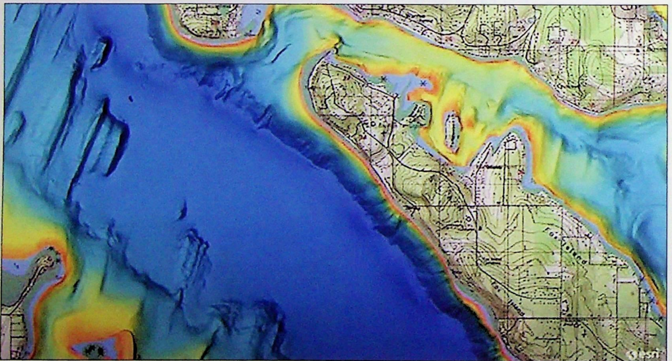
Figure 1.11 – BAG is now added over the sea area. The advantages of this data to confined water planning and execution are significant, particularly when considering and planning for bank effect, etc
