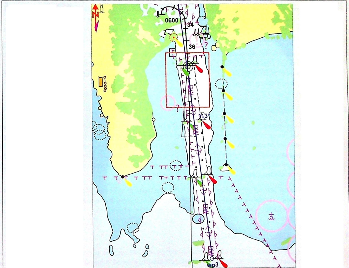
Figure 4.6 – Possible angular rotation shows incorrect alignment
