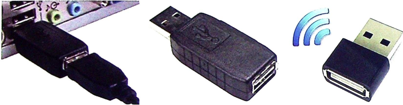
Figure 7.4 – Key loggers are openly available for purchase online. They can be connected to the WiFi or can use their own cellular data for live ‘monitoring’ ashore. The first keys usually typed into any computer are its passwords
