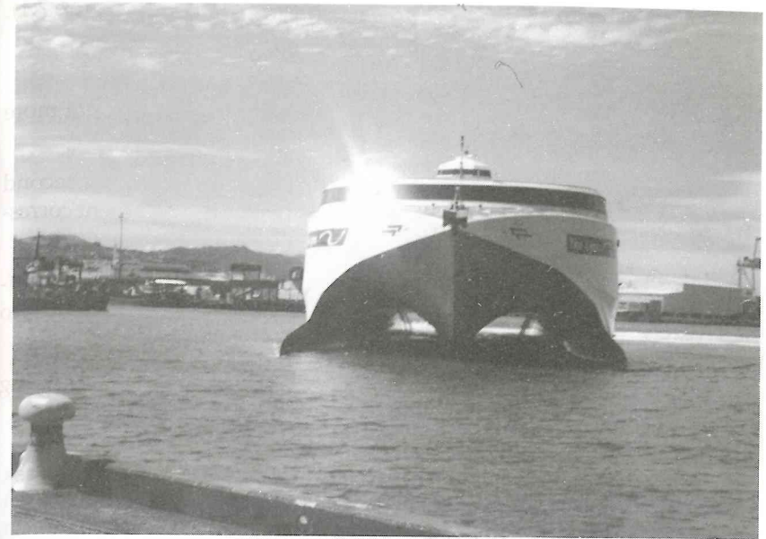
Fig. 7.3 The modern face of Ro-Pax type vessels. High-speed catamaran or tri-maran hulls with vehicle access from a stern ramp. Generally engaged on the short sea trades around the world, operating at service speeds up to 45 knots.
