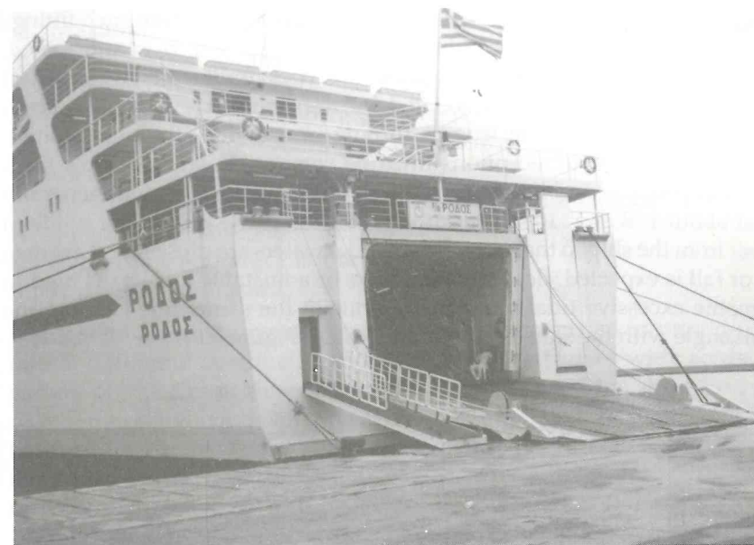
Fig. 7.6 Ro-Ro ferry example. Stern door/ramp access into the enclosed vehicle deck of a Ro-Pax ferry operating in the Mediterranean Sea.
