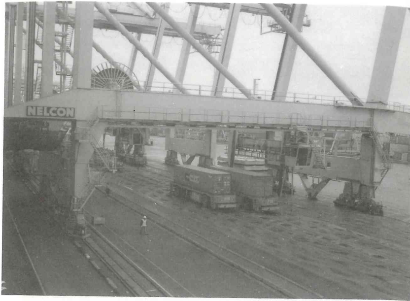
Fig. 8.24 Tracked shoreside 'gantry crane' for the loading of containers, semi-automatic, driverless transports deliver containers to its underside for loading aboard the container vessel.
