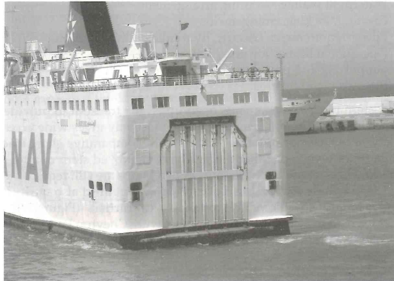
Fig. 7.10 Stern door of a Ro-Pax ferry seen in the stowed, closed position as she turns off the berth in the harbour at Tangier.
