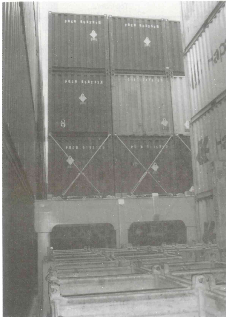
Fig. 8.21 Deck stowage and securing of container stack. The deck stow is seen in way of the edge of the pontoon hatch cover. The lashings are to the base, third tier container level by long bar (not shown). The second tier container level being secured by short bar lashings with the base containers locked to the pontoon.
