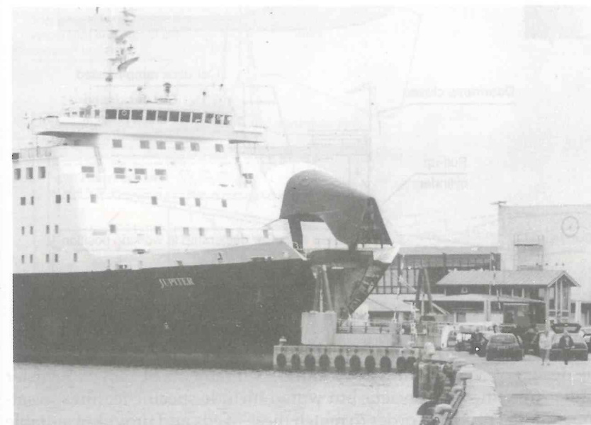
Fig. 7.7 The bow visor of the passenger vessel 'Jupiter' (since renamed) seen in the open position against the skyline. The bow visor fitted with a stern ramp
