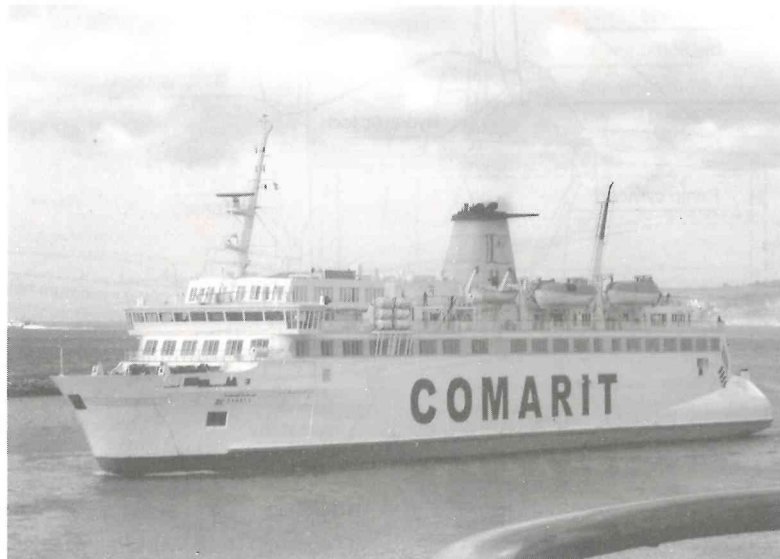
Fig. 7.11 The Ro-Pax ferry 'Sanasa' of the Comarit Ferry Group enters Tangier harbour. The vessel is fitted with a bow visor and stern/ramp door.
