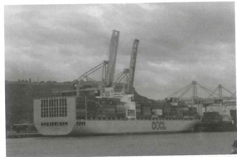
Fig. 8.13 The 'OOCL Shanghai' lies port side to the container terminal in Barcelona, Spain, after completing cargo loading with a full container load, the deck stack being at a six-tier height. The terminal 'gantry cranes' seen in the upright and clear position (the ship is not fitted with its own crange).
