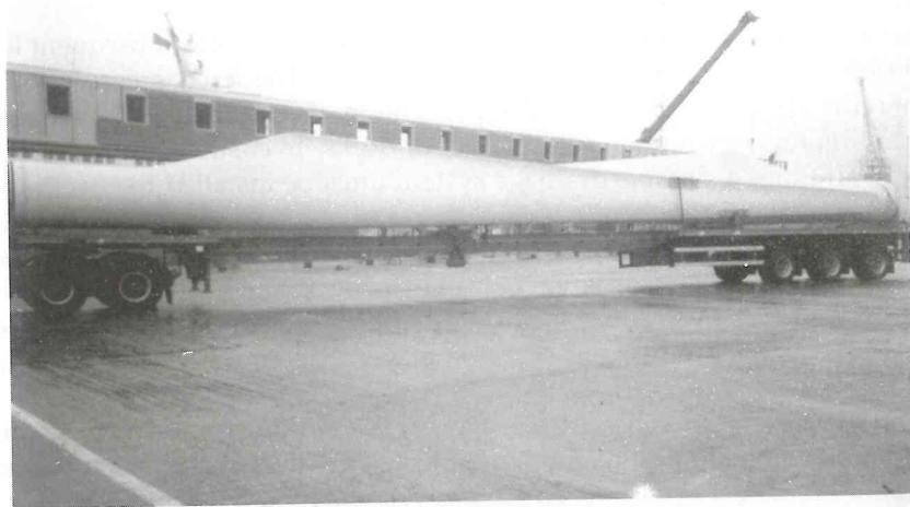
Fig. 7.17 Long load (sail for wind turbine) is loaded on adjustable stretch load trailer unit.
