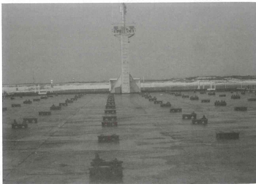
Fig. 8.16 The exposed container cargo deck of the 'Baltic Eider' seen with the container deck stool-securing points in uniform rows to form the basis of an even stow.
