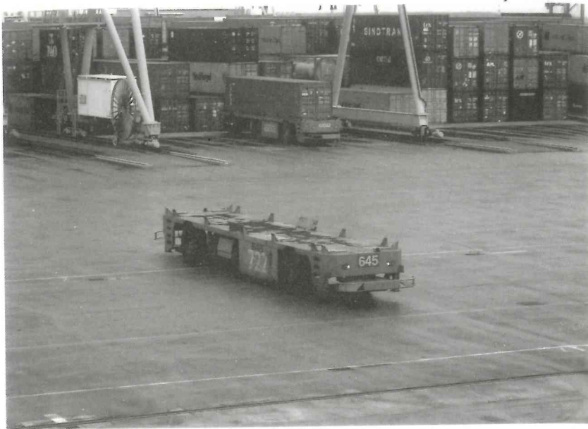
Fig. 8.29 Automated, driverless ground-handling transports deliver container units from the terminal stack to the underside of ship/shore gantry cranes.
