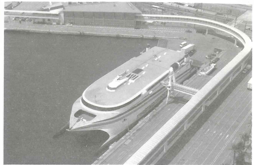
Fig. 7.25 The high-speed Ro-Pax catamaran vessel 'Millenium Dos' seen loading vehicles via the stern access, lying port side to the terminal in Barcelona, Spain.
