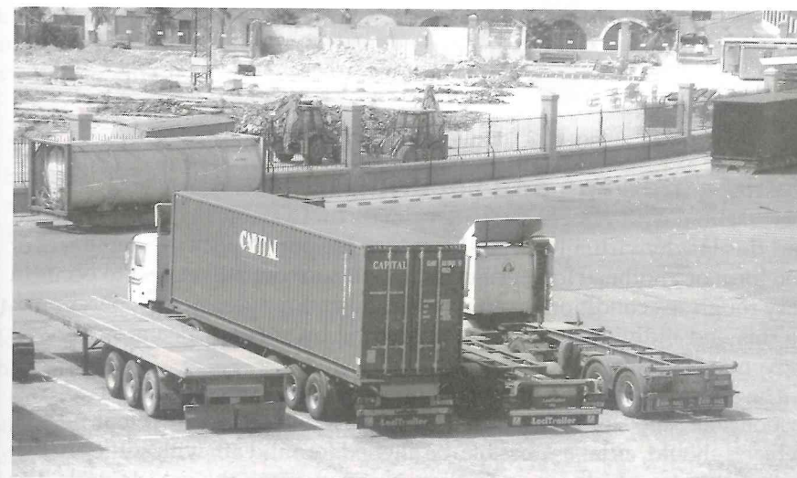
Fig. 7.18 Ro-Ro, unit types. Several Ro-Ro units on the quayside in Cadiz, Spain. From left to right: a flat-top trailer unit, a 40-ft container carrier, with two articulated container carriers on the end. A mobile tank container trailer unit is seen in the background.
