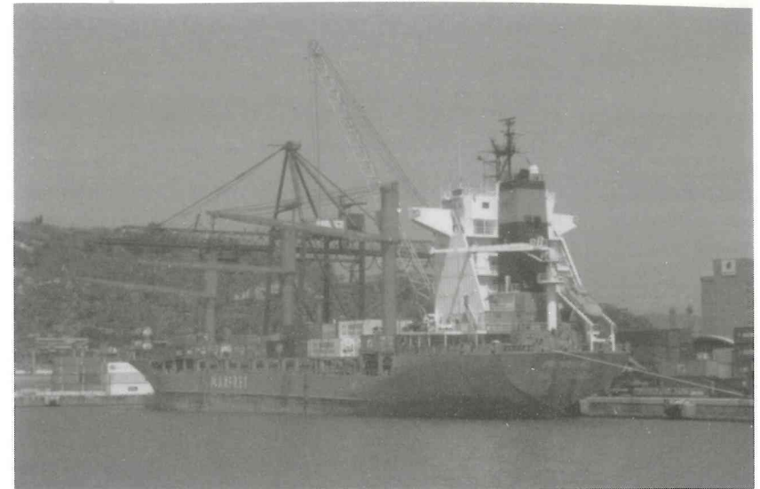
Fig. 8.27 A single gantry crane and a mobile dock side crane work the container cargo of the feeder container vessel 'Providence'. The ship's own container cranes are seen turned outboard to facilitate the shoreside loading systems in the port of Barcelona.
