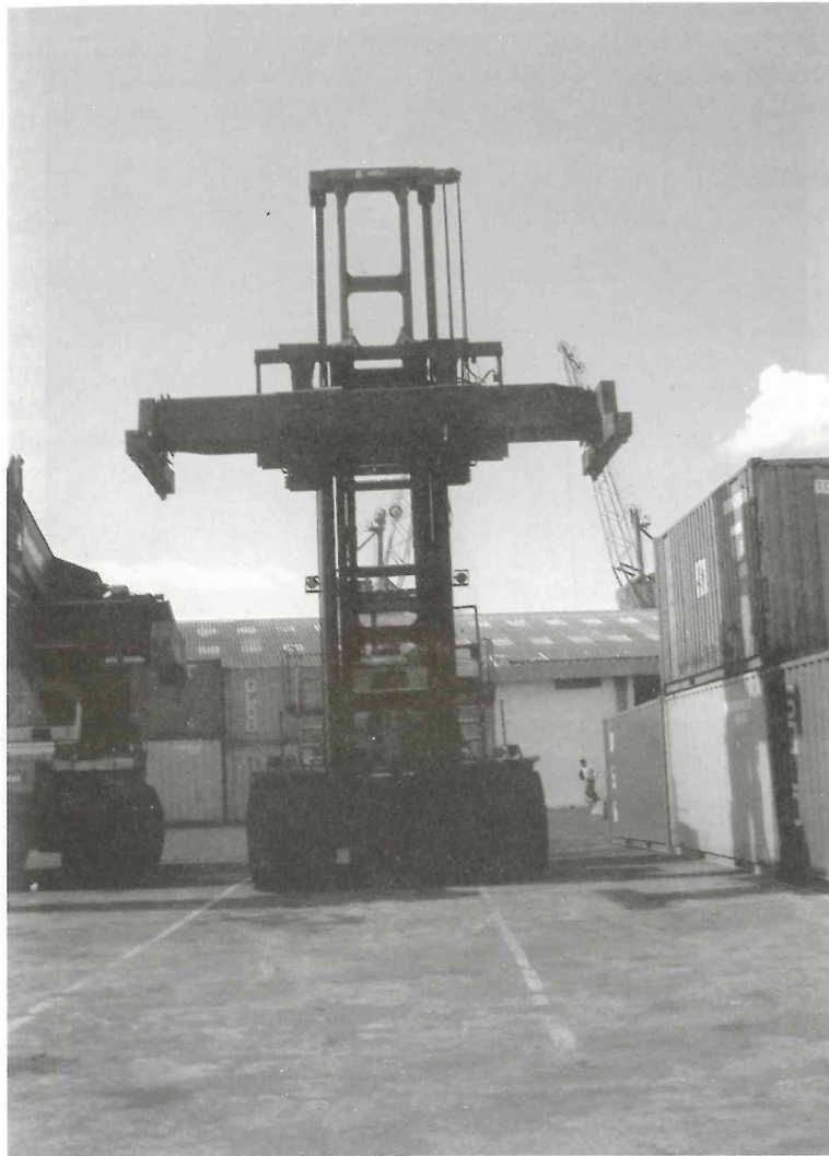
Fig. 8.35 Container terminal movement. Container transporter, with lift, transport, and stacking capability. A type of container karrilift based on the fork lift truck principle which is widely employed in container terminals worldwide.
