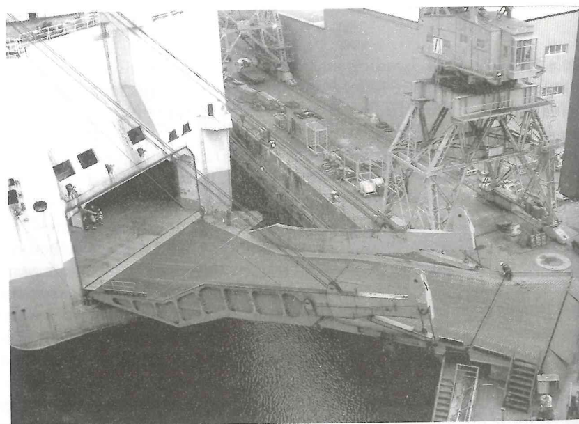
Fig. 7.30 A specialist unit load system. The angled quarter ramp and access point to vehicle decks of the above car carrier. These angled ramps have become a popular feature of car carrier vessels and are often employed with a midsection shell door ramp to improve the speed of load and discharge operations.
