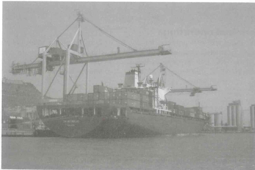
Fig. 8.26 The container gantry cranes discharge the vessel 'Zim Marseille' which lies port side to the container terminal in Barcelona, Spain.
