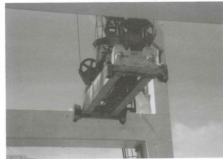
Fig. 8.9 The container spreader beam operates secured to the gantry crane travelling the length of the gantry jib to lift the containers on and off the vessel. The corners of the spreader beam are fitted with hinged droppable guides to ensure the beam locks can accurately locate the container corner recesses. The beam is also used to lift off pontoon hatch covers but when doing so does not deploy the hinged guides.
