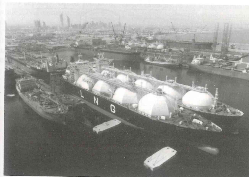
Fig. 5.26 Two LNG carriers lie alongside each other outside the Dubai Dry Dock Complex. These dedicated ships are prominent by the conspicuous cargo
