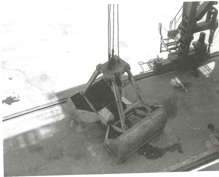
Fig. 4.14 Bucket mechanical grab seen in the open position on the quayside. The crane is configured so that the controlling crane driver can open and shut the grab by means of an operational wire to open and close the bucket arrangement.
