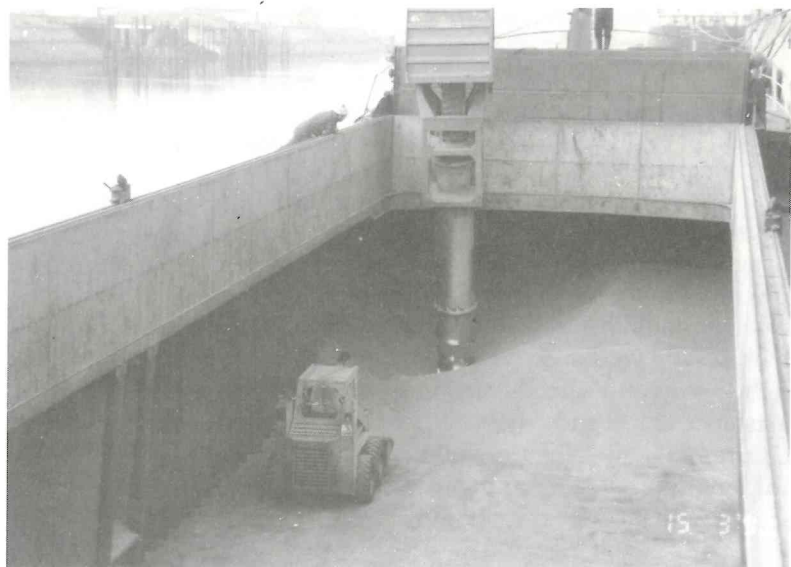
Fig. 4.13 A tractor is engaged in the tween deck of a vessel discharging cereals, to ensure that the suction of the grain elevator has access to all residuals of the cargo product.
