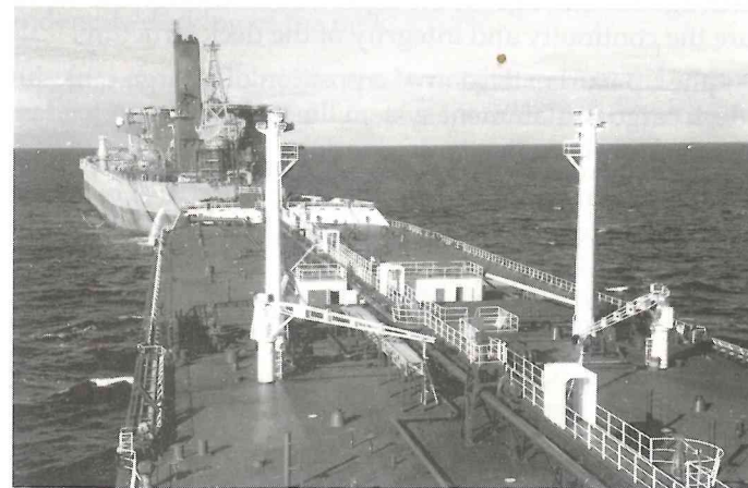
Fig. 5.3 Tanker approaches a floating storage unit (FSU). The pipeline-bearing boom of the FSU is seen in the vertical ready to be deployed once the tanker vessel has moored and connected to the stern of the FSU.
