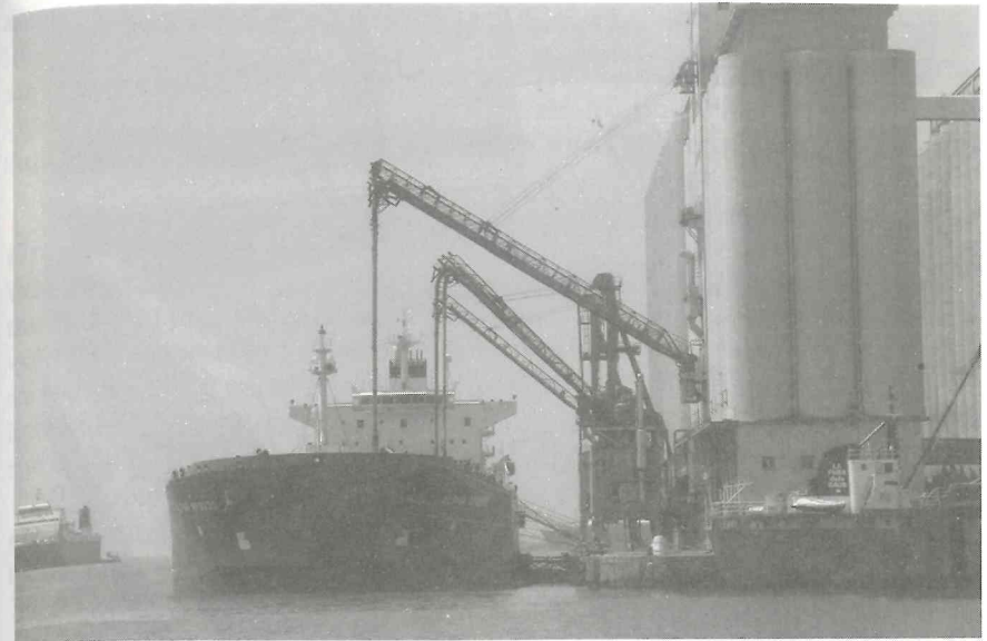
Fig. 4.10 The bulk carrier 'Alpha Afivos' lies port side to the grain silos in Barcelona. The grain elevators seen deployed into the ship's hold effecting discharge.
