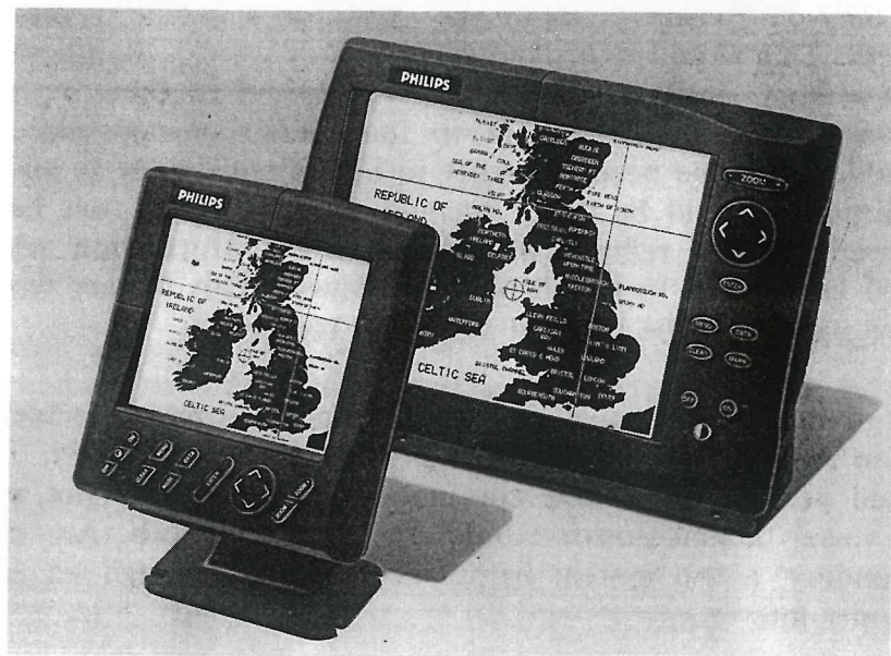
Electronic Chart Display Monitor can be free standing or incorporated into an integrated bridge system.
